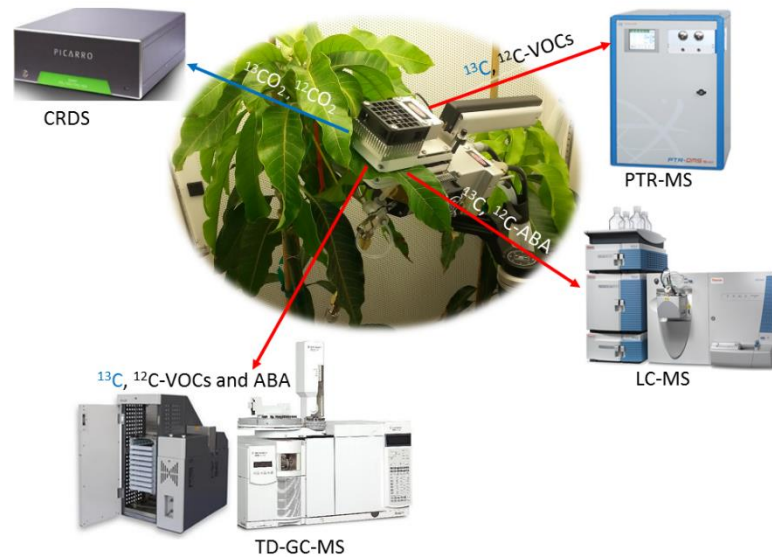
Figure 6. Example of a potential experimental instrumentation configuration for the quantification of ^{13}\text{C} -labeling analysis of volatile isoprenoids (isoprene and monoterpenes) and non-volatile isoprenoids (e.g. ABA and carotenoids) during photosynthesis under a ^{13}\text{CO}_2 atmosphere.
