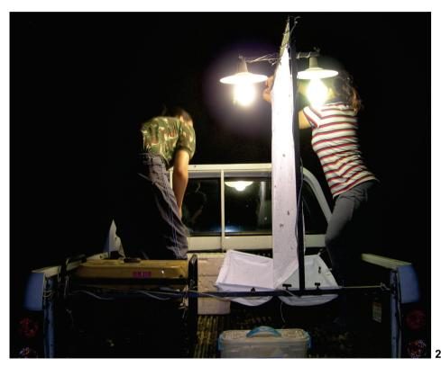
Figure 28. "mobile" light trap placed on a pick-up truck.
