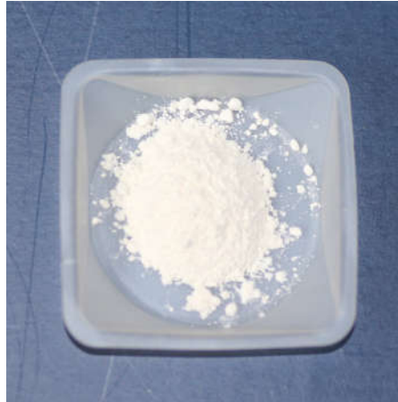
FIGURE 1: Amazonian metakaolin composed of 76% MK and 24% quartz.
