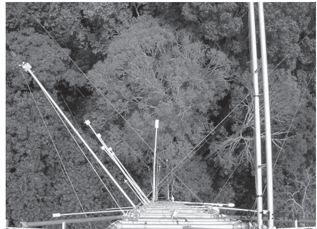
Figure 2. Profile of the nine cup anemometers installed in the Rebio-Jarú reserve's micrometeorological tower.
