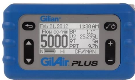
FIGURA 4: BOMBA DE VÁCUO PORTÁTIL - GILAIR PLUS PERSONAL AIR SAMPLING PUMP (1 – 5.000 CC/MIN).
