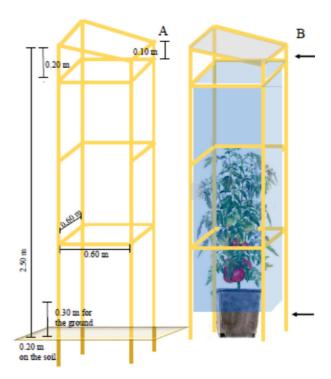
**Figure 1**: Schematic of greenhouse used for growing tomatoes with dimensions (A) and clear cover arrangement and plant location (B). The arrows indicate the openings for warm air outlet.
