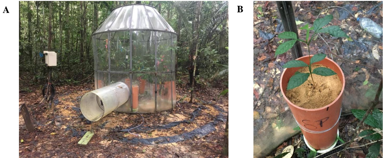
Figure S1 Photographs of the study area: A ) Photograph of an OTC, showing the steel-polypropylene structure and distribution of pots inside one of the OTCs B ) Photograph of a pot inside one of the open top chambers (OTCs), on day 160 of the experiment .
