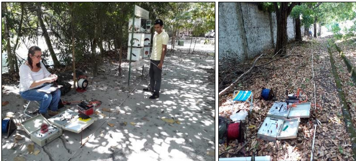
Figure 3. Photos of some points during the survey of electrical surveys carried out around the Lake area (VES1, VES2, VES3, VES4 and VES5) and the INPA Treatment Plant (VES6 and VES7).
