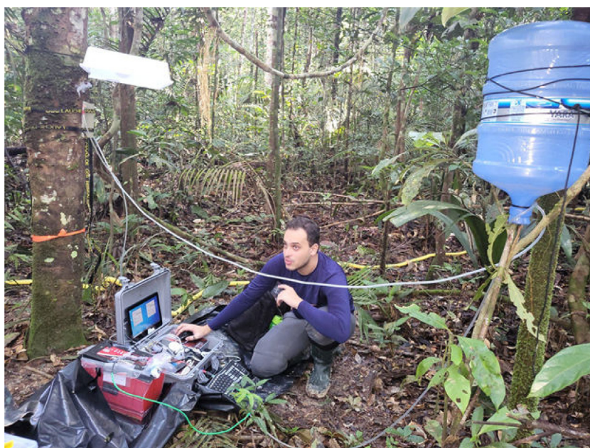
Fig. 5. Masters student Edson Augusto from the National Institute for Amazon Research (INPA) in Manaus, Brazil setting up a diurnal E_s data collection from a canopy tree in a remote central Amazon rainforest ecosystem.
