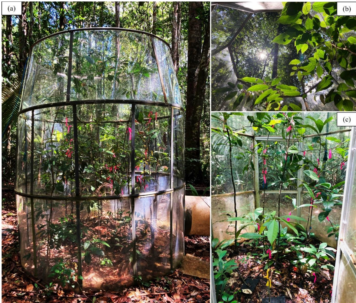
Figure S1 | Open top chamber structure. The figure illustrates (a) the design of an Open Top Chamber (OTC) structure, (b) the canopy open and (c) soil area used for investigating the effect of the increase in the CO 2 concentrations on understory plants. The OTC structure consists of a transparent polypropylene chamber with 3 m of height and 2.4 cm of diameter. Images: Maria Juliana, Flavia Santana.
